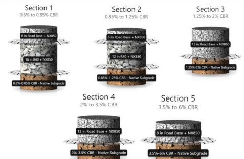
Menus of cross-sections incorporating InterAx geogrid.
