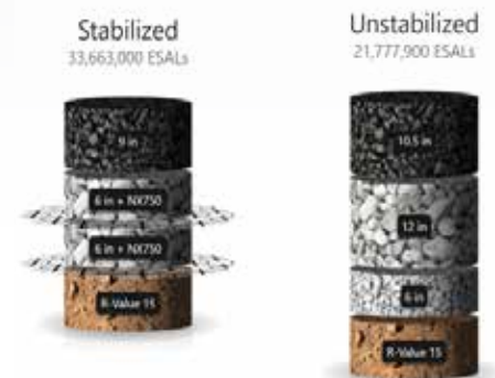
InterAx stabilized section (left) compared to an unstabilized section (right). This output from Tensar+ software shows the reduction in section thickness and increase in performance
